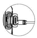
2) Charging with the micro USB slot at the bottom of the battery Remove the battery from the body of the radio, connect the data/charging cable to the micro USB slot at the bottom of the battery. The LED indicator can show the charging status.
